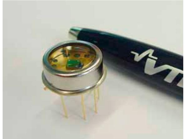
Miniature Fabry-Pérot Interferometer device made with MEMS technology (VTT). The principal transmission wavelength is tuned by changing the amount of space between the mirrors (Photo VTT)
