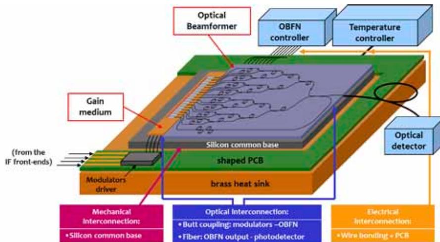
The design of the integrated optical beamforming system
