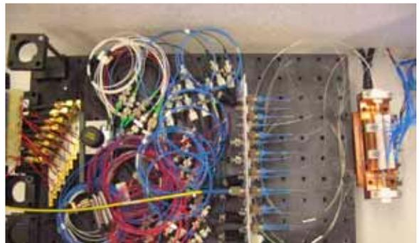
*The existing demonstrator, containing an older version of the optical chip (right) and off-the-shelf components with bulky glass-fibre cables (left). ‘Promis2Day’ will integrate all these components on a single photonic chip*
